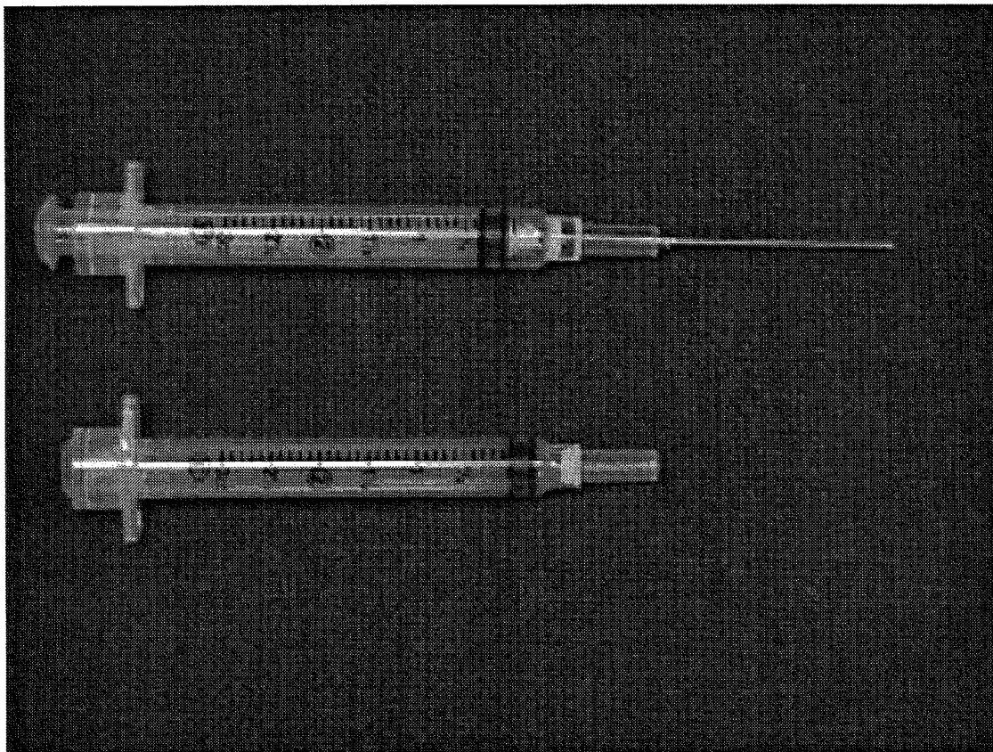
The VanishPoint ® Syringe before (top) and after (bottom) retraction.
