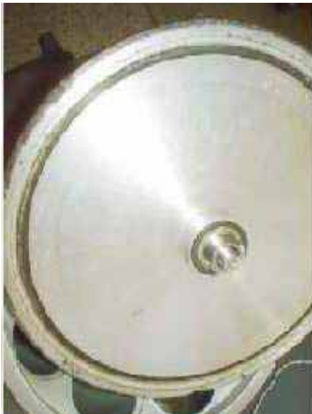
No containment is provided by this rotor or the bucket safety covers because O-rings were either not installed or replaced as required.
