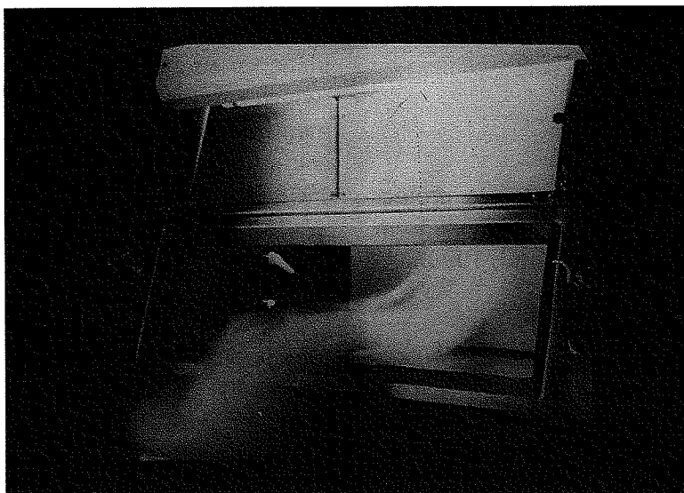
FIGURE 2 Smoke being swept away in a Class I Biological Safety Cabinet.
